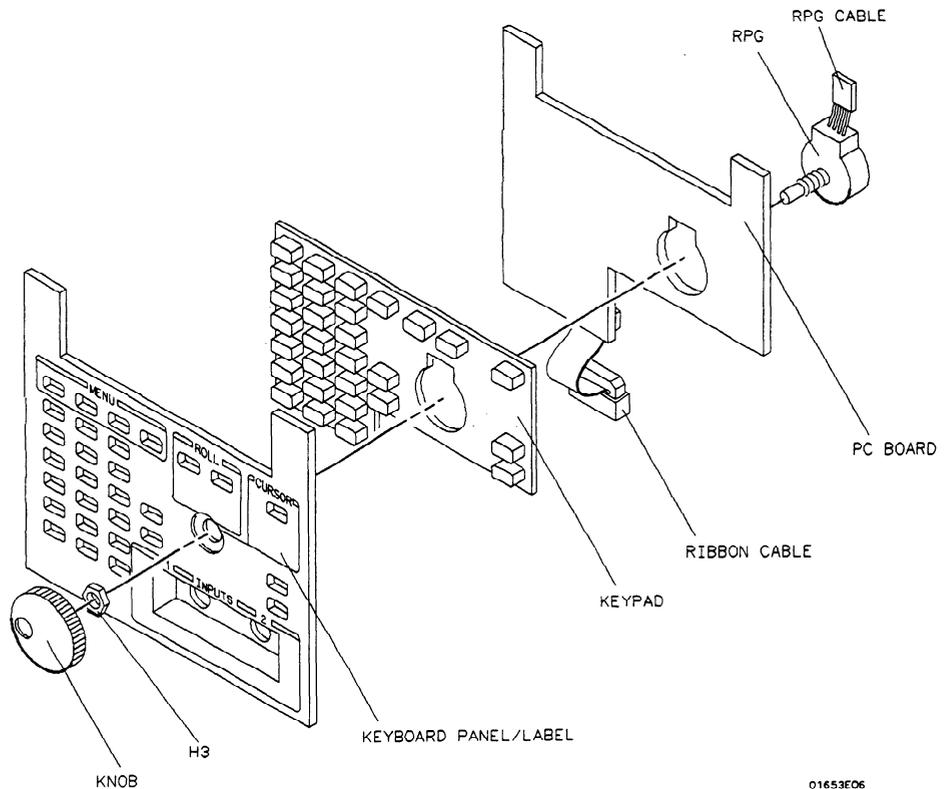
**Figure 6D-5. Exploded view of the Keyboard Assembly**
