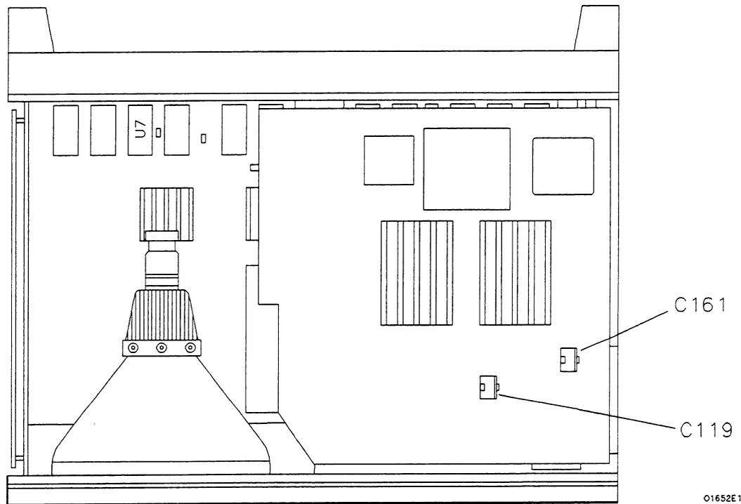
**Figure 4-6. High-Frequency Pulse Adjustments**
