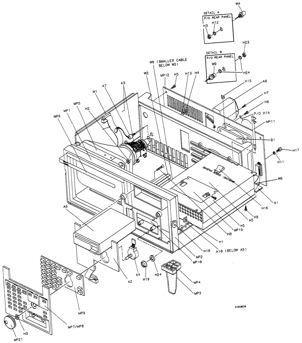
Figure 5-1. HP 1652B/1653B Exploded View
